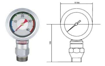
1280 Series mud pressure gauges standard with a 2" male BSP (other sizes also are available). It has a large liquid filled case for easy viewing at distances of more than 60 feet. This style of gauge has been in service on mud pumps and standpipes for decades and has proven to be a low cost, reliable gauge that withstands the rigors of oilfield use.
