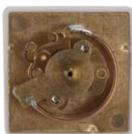
Built-in Pressure Gauge 1181F type with open/close cover, minimum-maximum pointer
